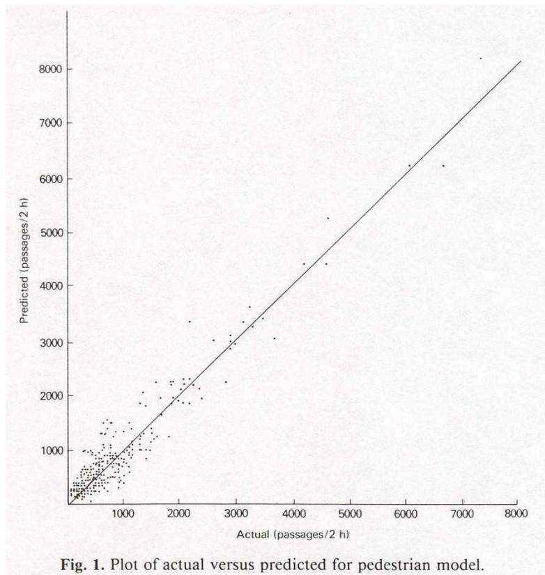
Fig. 1. Plot of actual versus predicted for pedestrian model.
